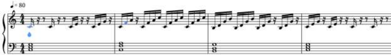
Figure 3. Sonification of a continuous data signal where the differences in the input signal are encoded into the number of sixteenth notes present in an arpeggio starting from the bottom.
